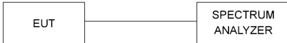
Figure 1 - Bandwidth Measurements Test Setup
