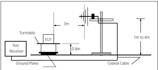
(c) For radiated emissions above 1000MHz
