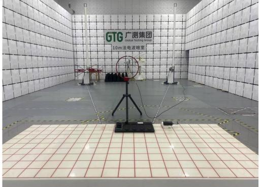
**30MHz-1GHz Radiated Emission**
