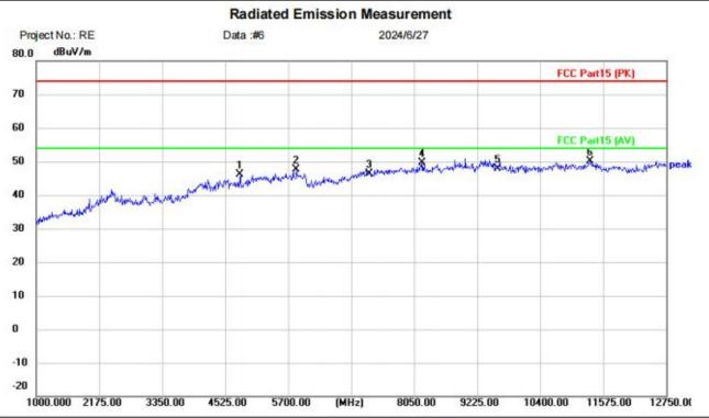
Site Polarization: Vertical Temperature: (C) Power: Humidity: %RH
