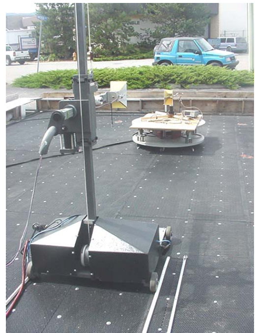
Photograph B.7-4 - Horn Substitution Setup
