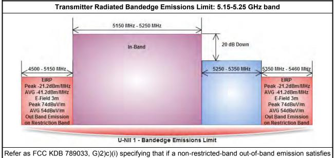
Refer as FCC KDB 789033, G)2)c)(i) specifying that if a non-restricted-band out-of-band emission satisfies both the average and peak limits of 15.209, it is not required to satisfy the -27 dBm or -17 dBm peak emission limit. Reason for change: to ensure that emission requirements in the non-restricted bands are not more stringent than those in the restricted bands.
