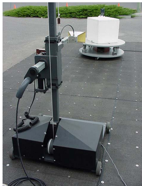
Photograph C.7-4 - Dipole Substitution Setup
