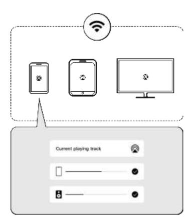
The WiiM Mini can play AirPlay 2 audio, which allows you to quickly stream audio from your Apple device to the external speaker or multiple speakers.
