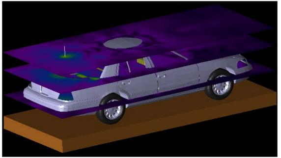
The equivalent power density (S) is computed from the E-field. The following table reports the E-field values computed by  $XFDTD^{TM}$  at the three locations, and the corresponding power density.
