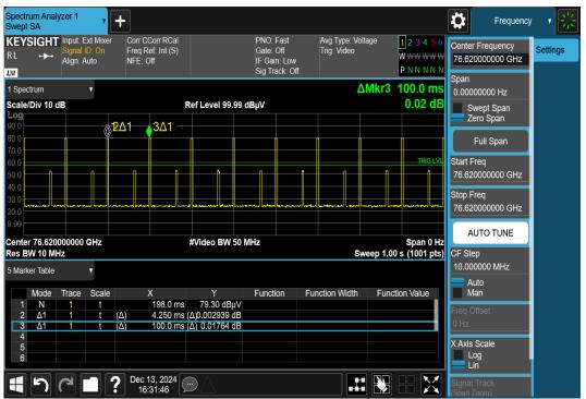
Note: The signal at the second altitude is another radar signal, so this signal is not evaluated.
