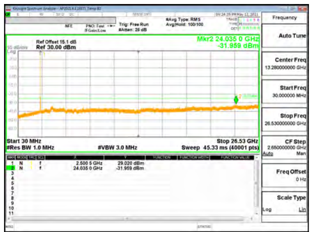
5G NR n7 10MHz BPSK Low Channel RB1-0
