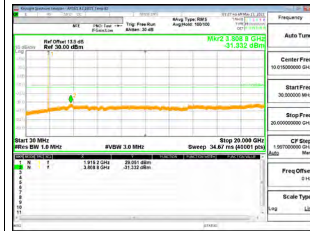
5G NR n25 5MHz BPSK High Channel RB1-24
