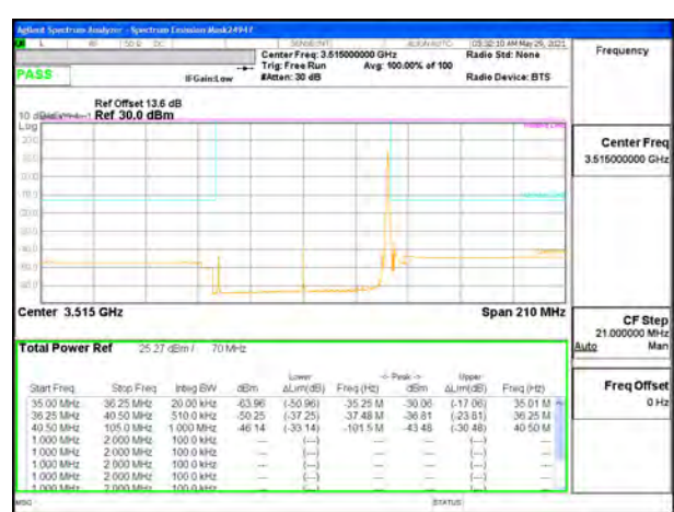
5G NR n77 70MHz BPSK High Channel RB1-188
