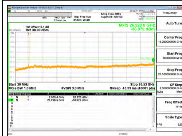
5G NR n7 40MHz BPSK High Channel RB1-215
