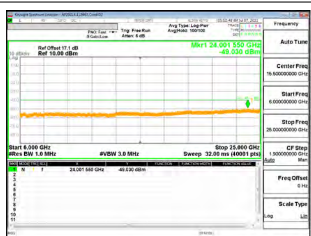
5G NR n30 5MHz BPSK Low Channel RB1-0 (6G to 25G)
