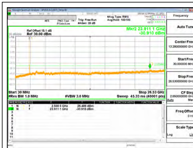
5G NR n7 25MHz BPSK Low Channel RB1-0
