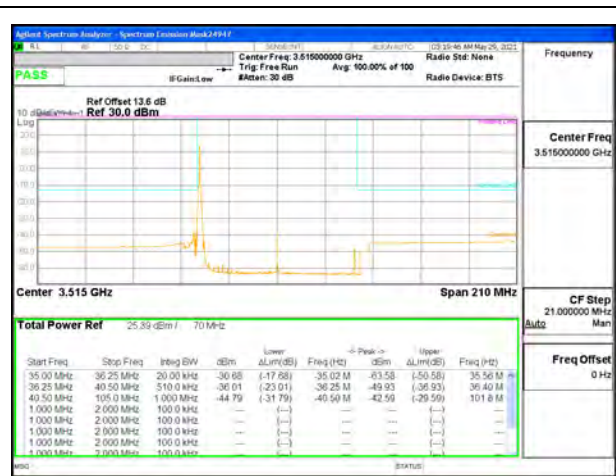
5G NR n77 70MHz BPSK High Channel RB1-0
