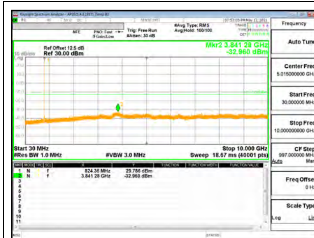
5G NR n5 5MHz BPSK Low Channel RB1-0
