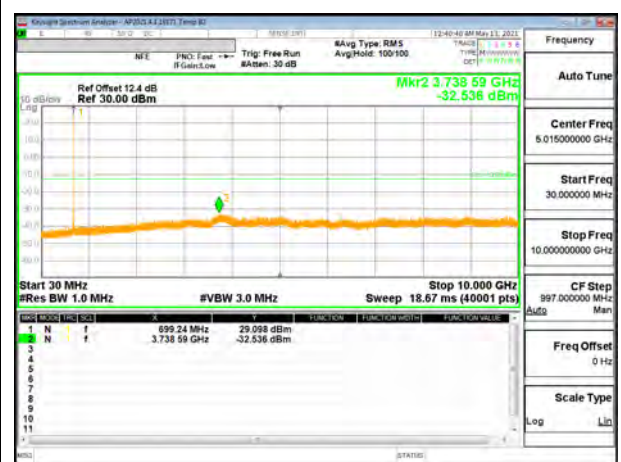
5G NR n12 10MHz BPSK Low Channel RB1-0
