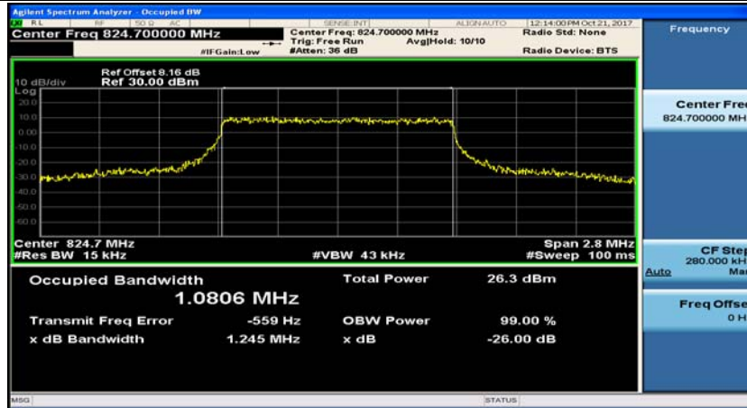
(Channel Bandwidth: 1.4 MHz)_LCH_16QAM_6RB#0
