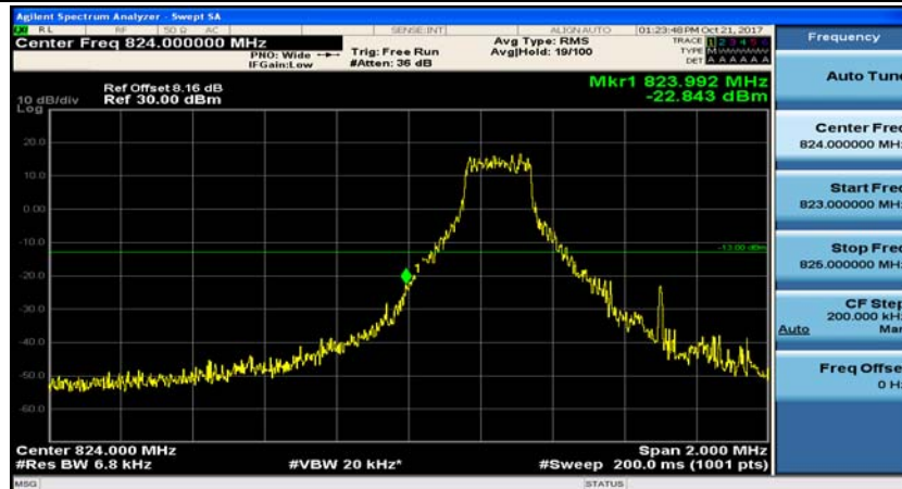
(Channel Bandwidth: 1.4 MHz)_LCH_QPSK_1RB#3
