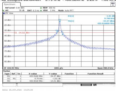
99% occupied bandwidth = 20.38kHz < 433.92 MHz\* 0.25%= 1.08 MHz
