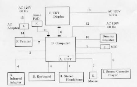
Symbols or numbers assigned to equipment or cables on this diagram are corresponded to the symbols or numbers assigned to equipment or cables on tables in Sections 3 to 5.
