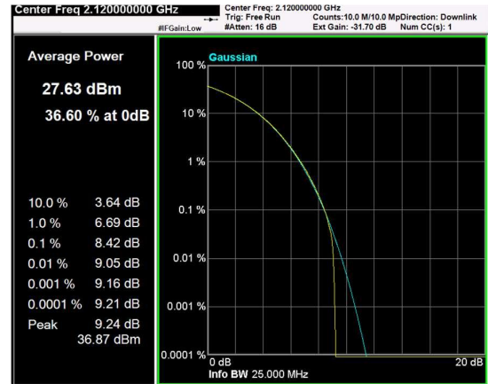
Channel: BOTTOM, Modulation: 16QAM, BW=20MHz, CCDF
