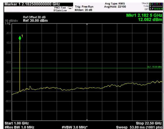
Channel: TOP, Modulation: QPSK, BW=10MHz, Range: Upper
