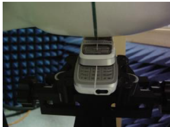
Fig.9 Photograph of the Left Hand Side Tilt ,on status
