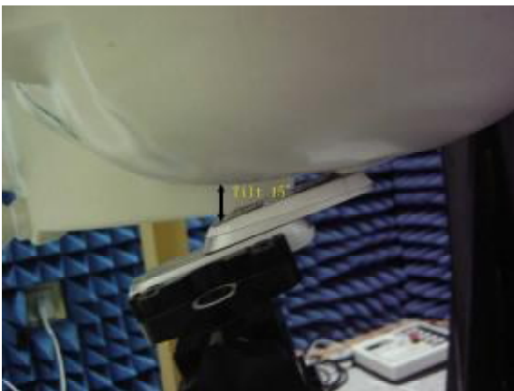
Fig.9 Photograph of the Left Hand Side Tilt ,on status
