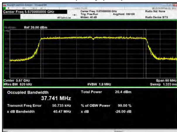
U-NII-2C, 802.11ax HE40 Carrier frequency (MHz): 5710
