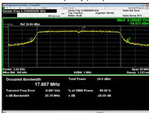
U-NII-1, 802.11n HT20 Carrier frequency (MHz): 5240
