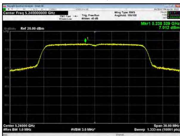
U-NII-1, 802.11ac VHT20, Channel No.: 48
