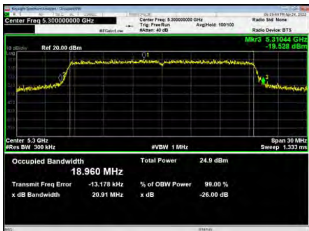
U-NII-2A, 802.11ax HE20 Carrier frequency (MHz): 5320
