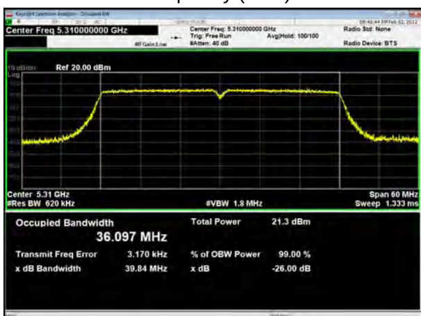
U-NII-2A, 802.11n HT40 Carrier frequency (MHz): 5310
