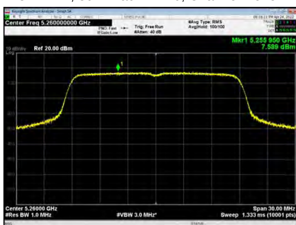
U-NII-2A, 802.11ac VHT20, Channel No.: 60
