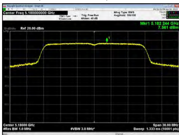
U-NII-1, 802.11ac VHT20, Channel No.: 40
