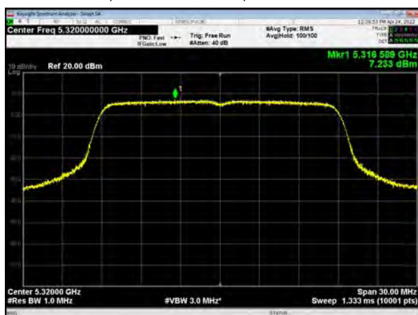
U-NII-2A, 802.11ac VHT20, Channel No.: 52
