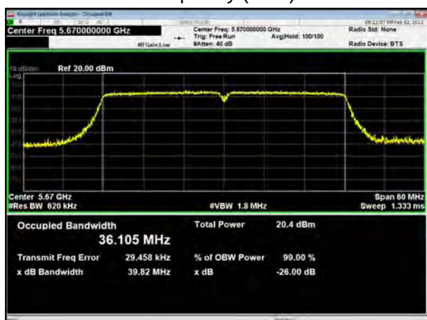
U-NII-2C, 802.11n HT40 Carrier frequency (MHz): 5670
