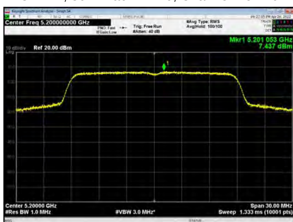
U-NII-1, 802.11ac VHT20, Channel No.: 48
