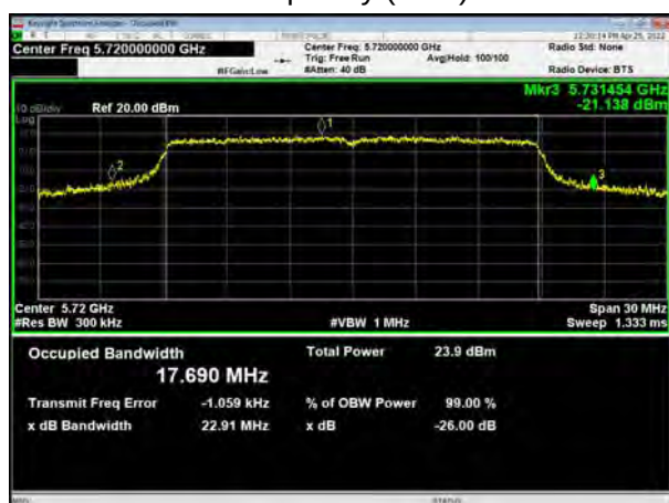
U-NII-2C, 802.11n HT20 Carrier frequency (MHz): 5720
