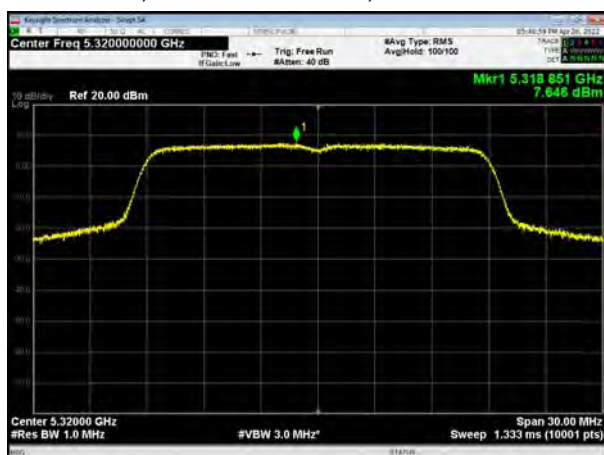
U-NII-2A, 802.11ac VHT80, Channel No.: 58
