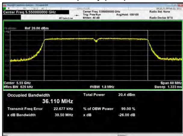
U-NII-2C, 802.11n HT40 Carrier frequency (MHz): 5670
