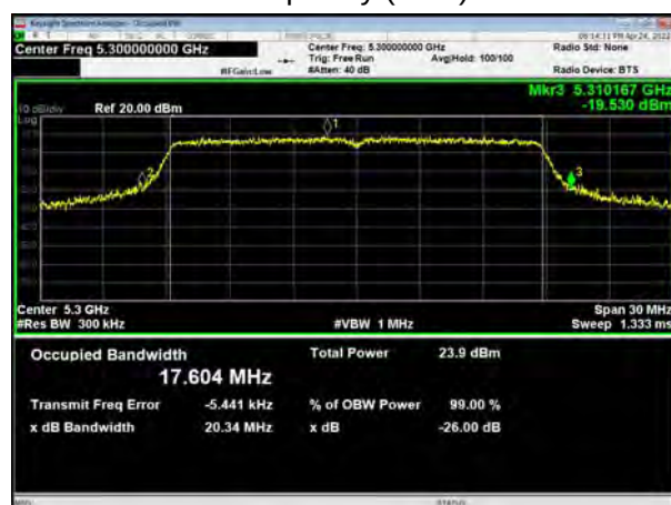
U-NII-2A, 802.11n HT20 Carrier frequency (MHz): 5300
