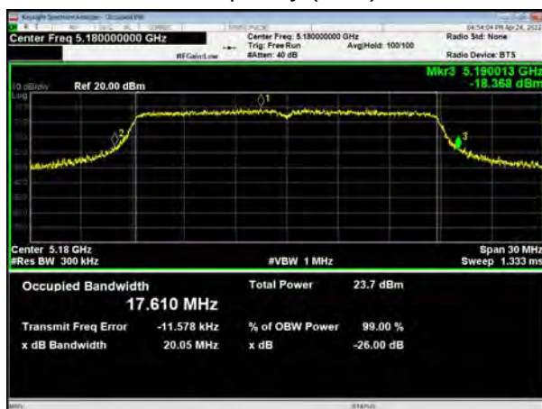
U-NII-1, 802.11n HT20 Carrier frequency (MHz): 5200
