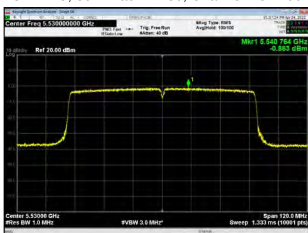
U-NII-2C, 802.11ac VHT80, Channel No.: 138
