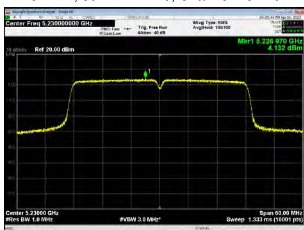
U-NII-1, 802.11ac VHT40, Channel No.: 38
