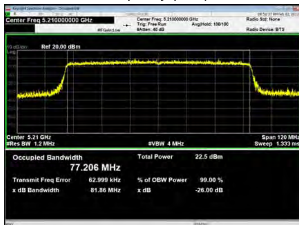
U-NII-2A, 802.11n HT20 Carrier frequency (MHz): 5260
