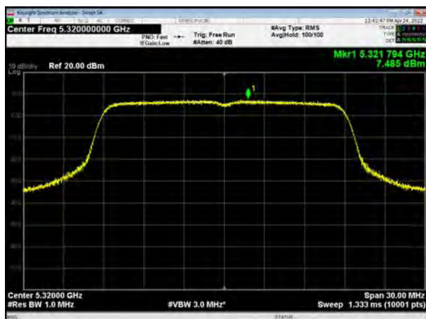
U-NII-2A, 802.11ac VHT80, Channel No.: 58
