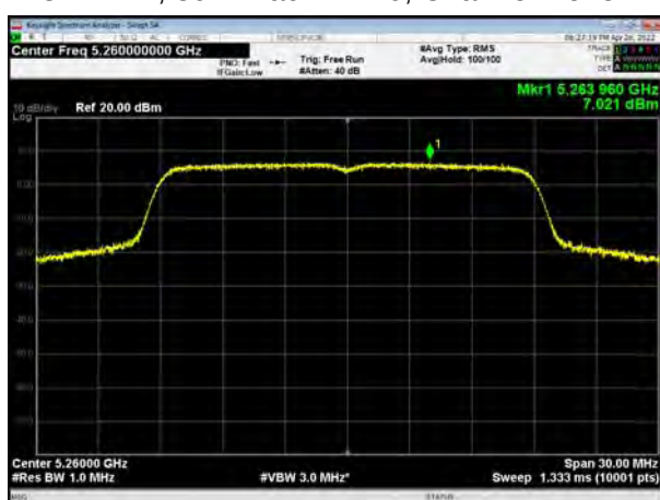
U-NII-2A, 802.11ac VHT20, Channel No.: 60
