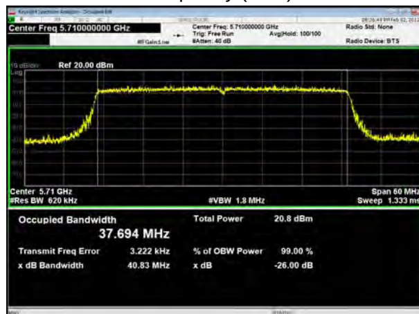
U-NII-2C, 802.11ax HE80 Carrier frequency (MHz): 5690
