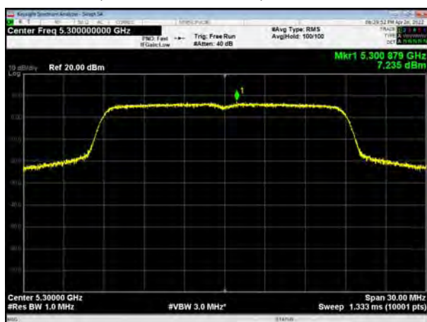
U-NII-2A, 802.11ac VHT20, Channel No.: 60
