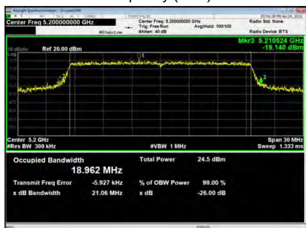
U-NII-1, 802.11ax HE20 Carrier frequency (MHz): 5200
