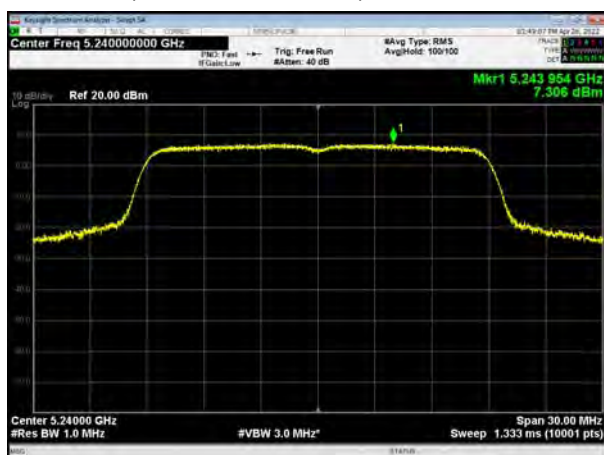
U-NII-1, 802.11ac VHT20, Channel No.: 48
