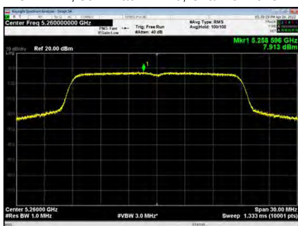
U-NII-2A, 802.11ac VHT20, Channel No.: 60
