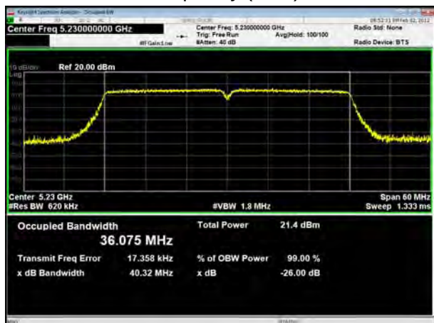
U-NII-1, 802.11ax HE20 Carrier frequency (MHz): 5180
