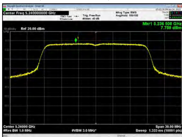
U-NII-1, 802.11ac VHT20, Channel No.: 48
