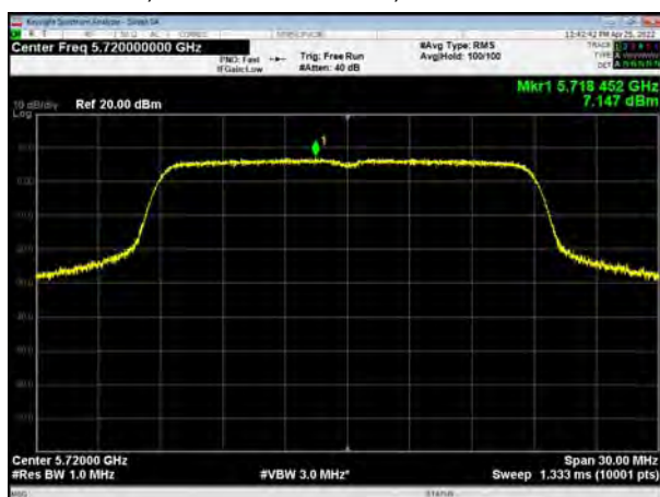
U-NII-2C, 802.11ac VHT80, Channel No.: 106
