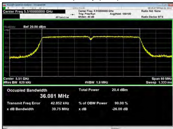
U-NII-2C, 802.11n HT40 Carrier frequency (MHz): 5550
