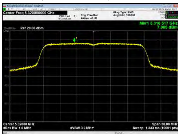
U-NII-2A, 802.11ac VHT80, Channel No.: 58
