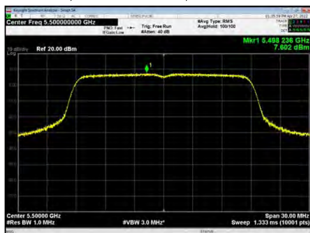
U-NII-2C, 802.11ac VHT20, Channel No.: 116
