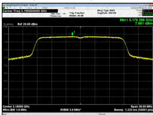
U-NII-1, 802.11ac VHT20, Channel No.: 40
