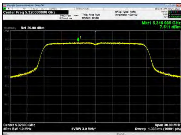
U-NII-2A, 802.11ac VHT80, Channel No.: 58
