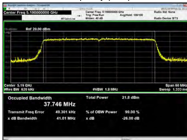
U-NII-1, 802.11ax HE40 Carrier frequency (MHz): 5230
