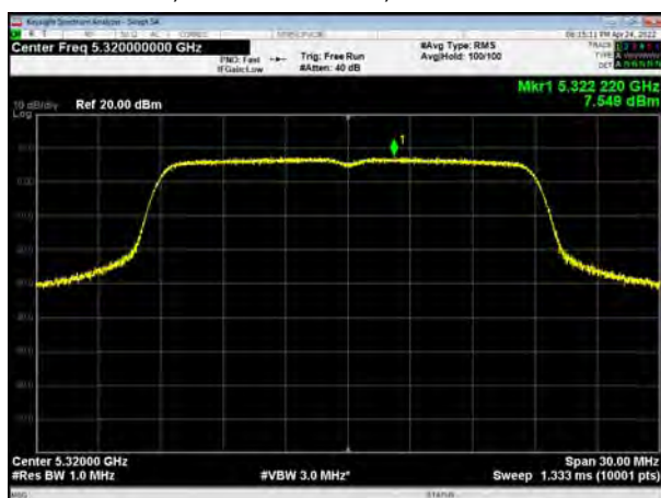
U-NII-2A, 802.11ac VHT20, Channel No.:52
