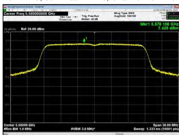
U-NII-2C, 802.11ac VHT20, Channel No.: 140
