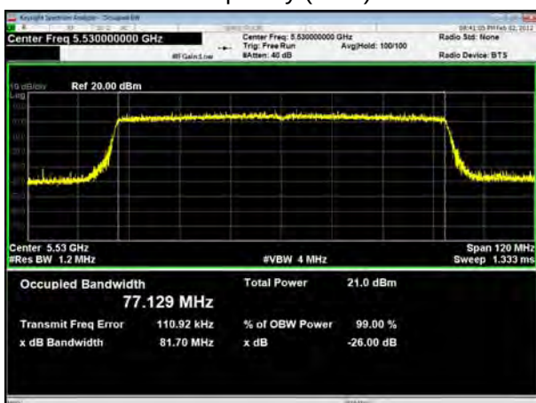
U-NII-2C, 802.11ax HE80 Carrier frequency (MHz): 5530
