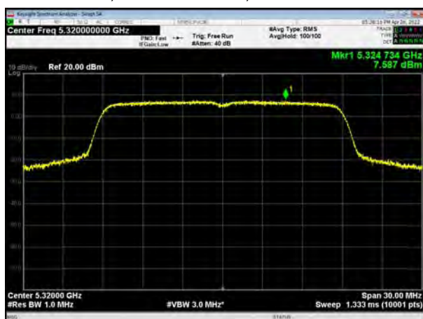
U-NII-2A, 802.11ac VHT20, Channel No.: 52
