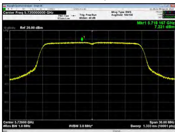
U-NII-2C, 802.11ac VHT80, Channel No.: 106
