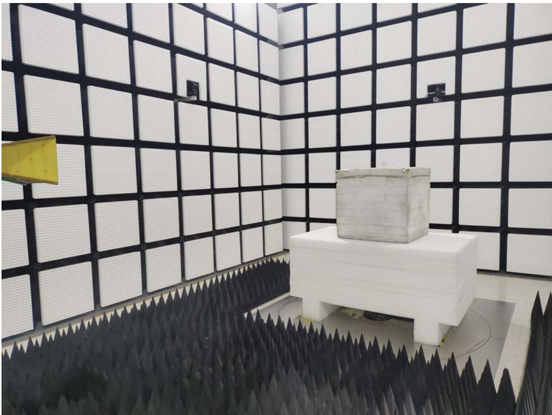
Radiated Emission Above 1GHz View EM320-TH-915M
