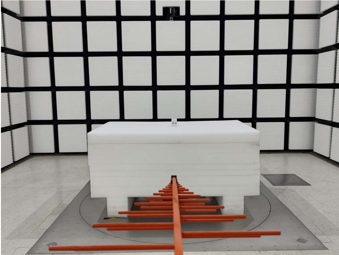
Radiated Emission Above 1GHz View EM320-TH-915M
