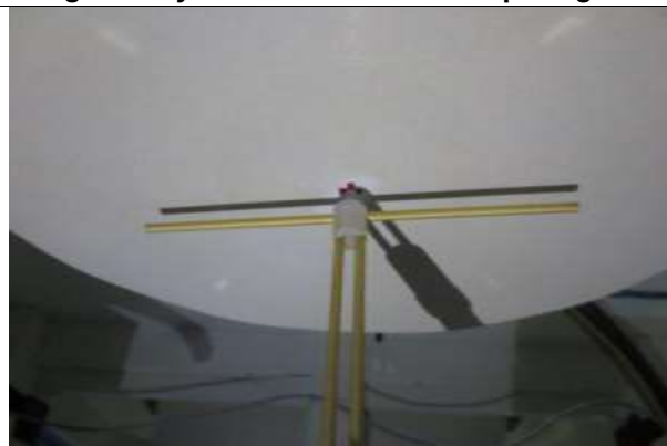
Fig.10.2 Photo of Dipole setup
