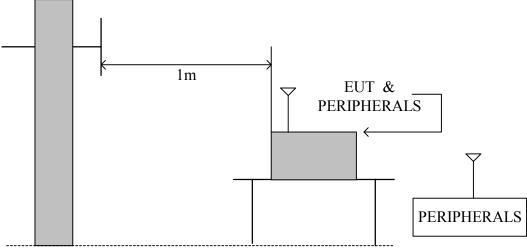
Antenna Elevation Variable
