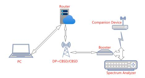
UUT Connect to certified CBSD by RF cable, the companion device is a end user device
