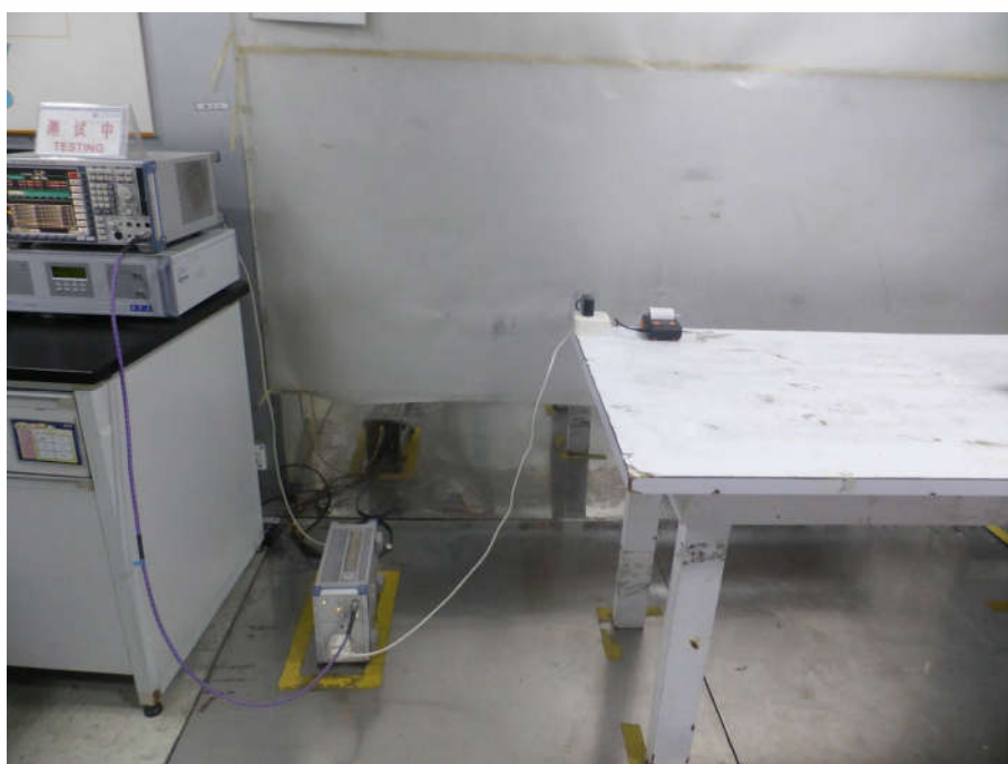
Conducted Emissions Test Setup
