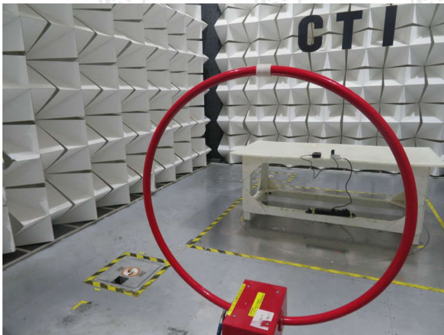
Radiated spurious emission Test Setup-1(Below 30MHz)
