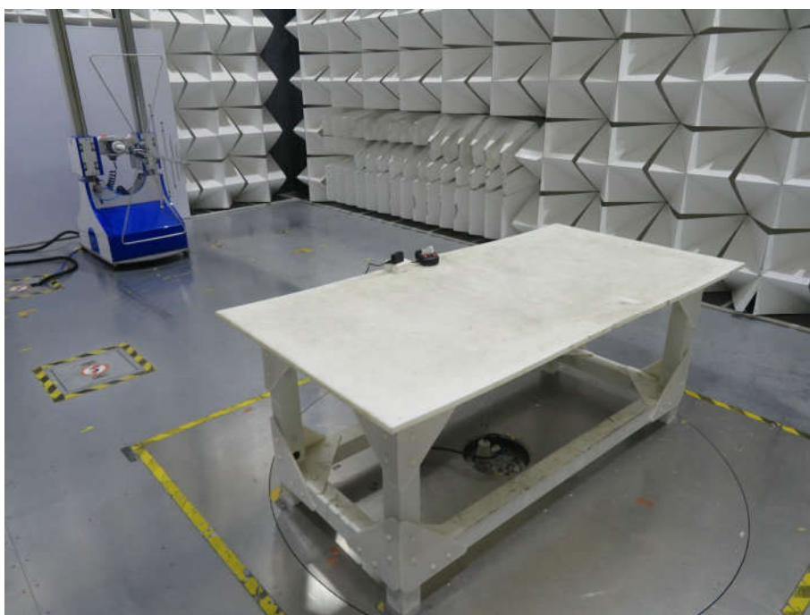
Radiated spurious emission Test Setup-2(Below 1G)
