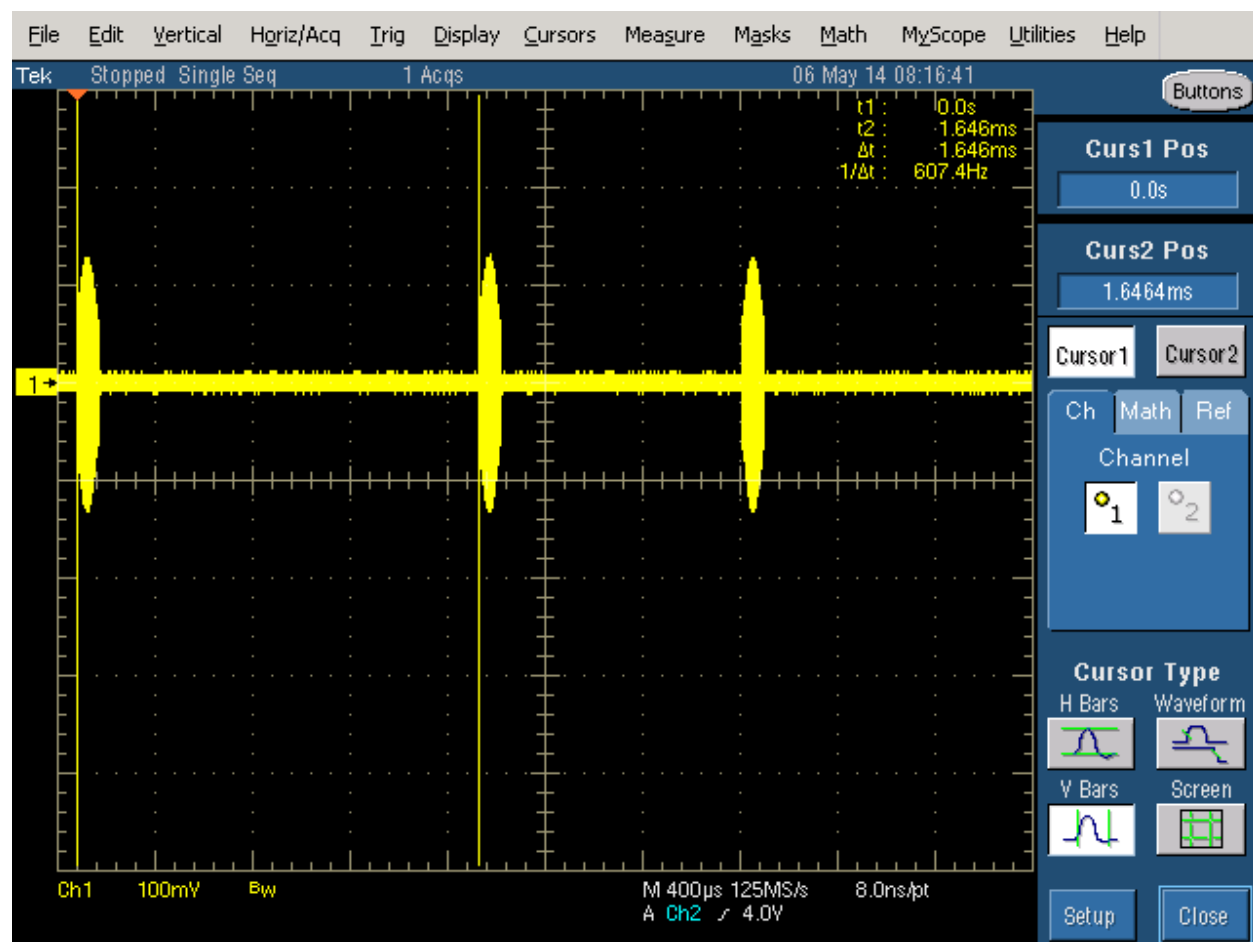
Figure 8 - FCC Type 5 Radar (burst with three pulses, 1650 µs first period)
