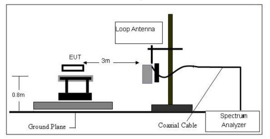
(B) Radiated Emission Test-Up Frequency 30MHz~1GHz
