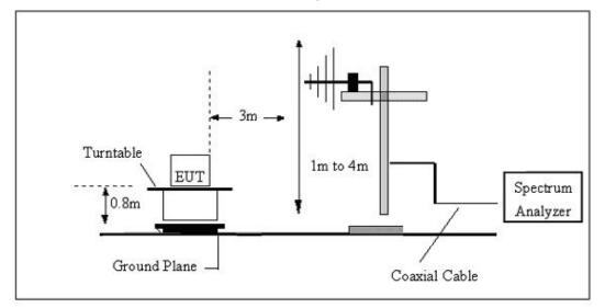
(C) Radiated Emission Test-Up Frequency Above 1GHz
