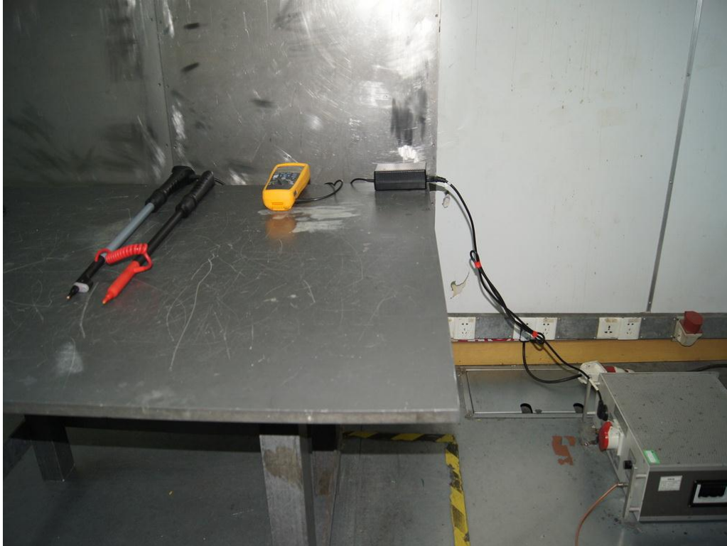
Photograph 1: Set-up for Conducted Emission
