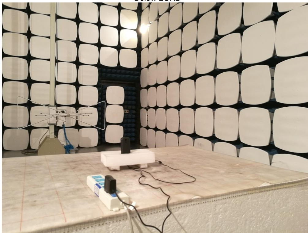
Radiated Spurious Emission Below 1GHz
