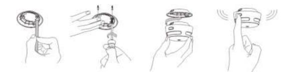
NOTE: Before installation, it is recommended to test the interconnected smoke alarms in different rooms where you intend to install these alarms to ensure that they are within the transmission range.
