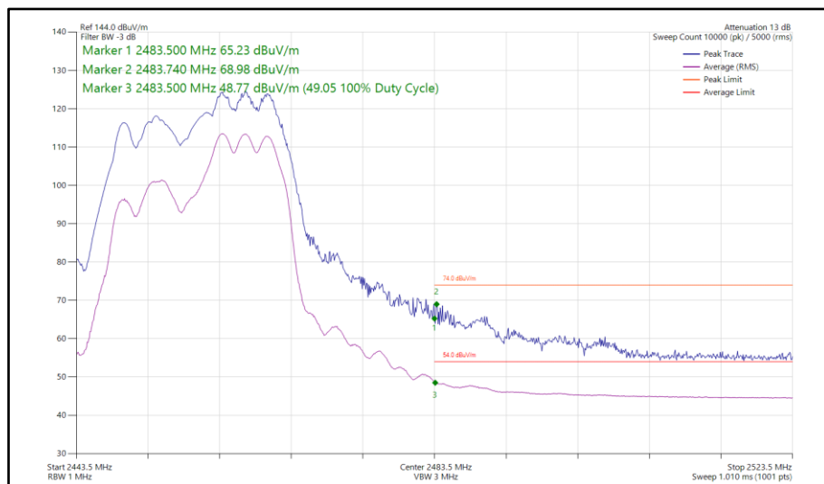
Figure 119 - 802.11ax HE20, RU 106-54, CDD, Core 0 - Core 1 - 2457 MHz Band Edge Frequency 2483.5 MHz
