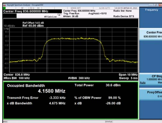
(Plot E2: WCDMA 850MHz Channel = 4183 Occupied bandwidth)
