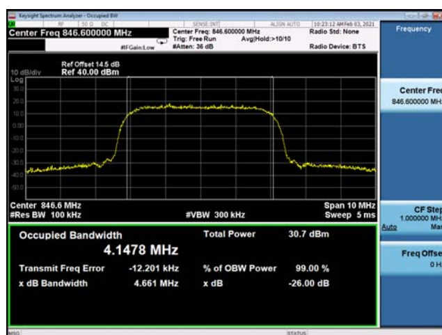
(Plot E3: WCDMA 850MHz Channel = 4233 Occupied bandwidth)
