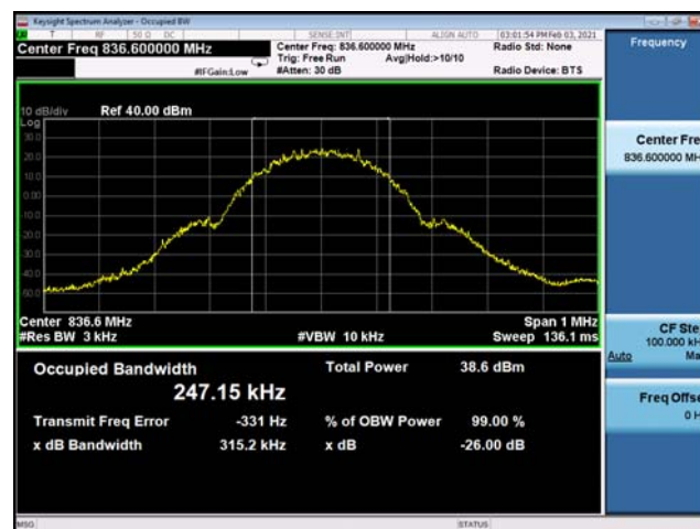
(Plot A2: GSM 850MHz Channel = 190 Occupied bandwidth)
