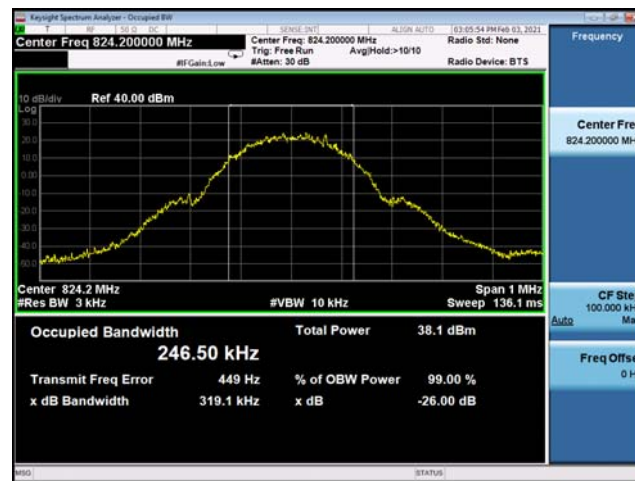
(Plot A1: GSM 850MHz Channel = 128 Occupied bandwidth)
