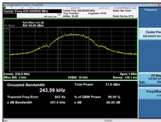
(Plot C2: EDGE 850MHz Channel = 190 Occupied bandwidth)
