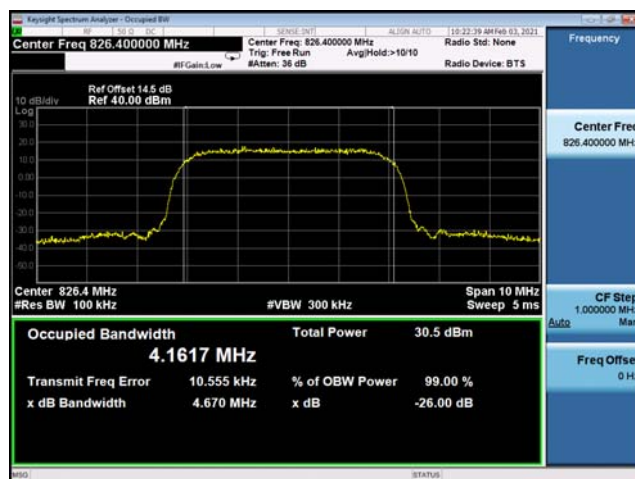
(Plot E1: WCDMA 850MHz Channel = 4132 Occupied bandwidth)
