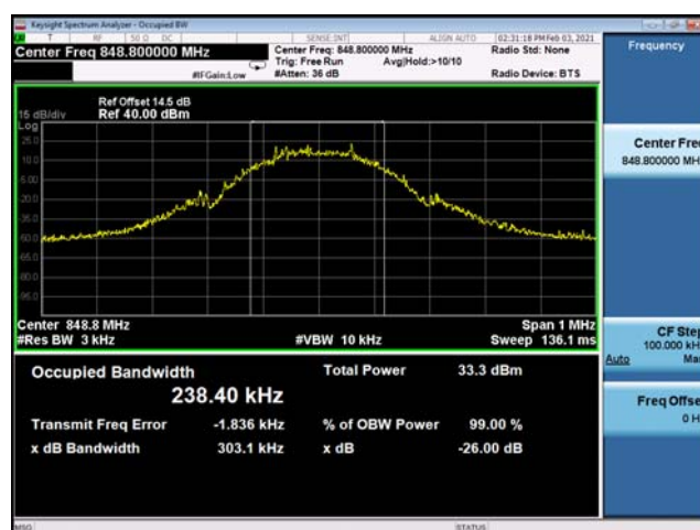
(Plot C3: EDGE 850MHz Channel = 251 Occupied bandwidth)
