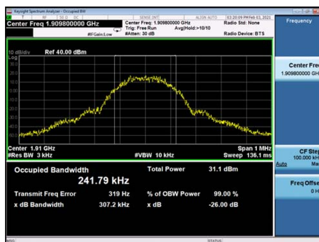
(Plot D3: EDGE 1900MHz Channel = 810 Occupied bandwidth)
