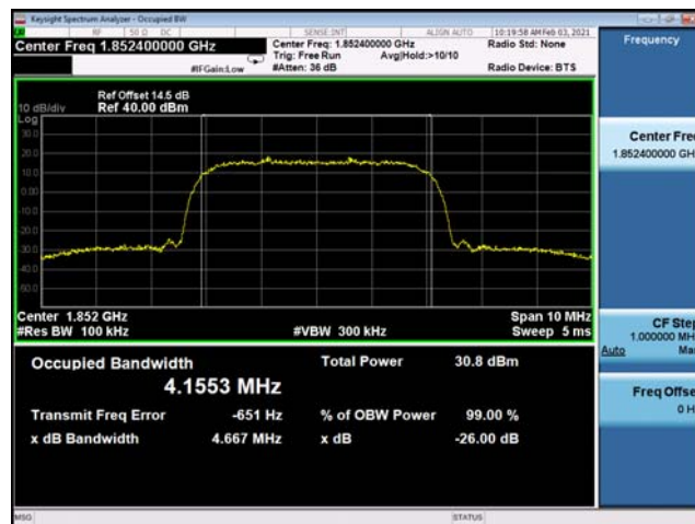
(Plot F1: WCDMA 1900MHz Channel = 9262 Occupied bandwidth)
