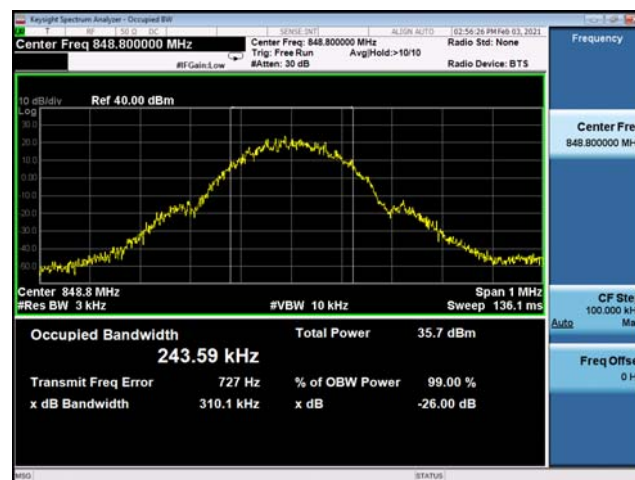
(Plot A3: GSM 850MHz Channel = 251 Occupied bandwidth)
