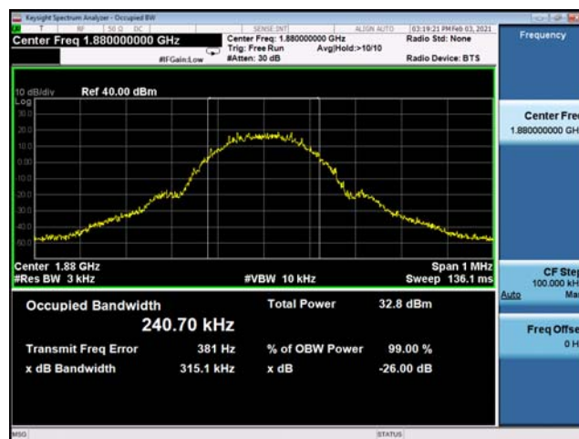
(Plot D2: EDGE 1900MHz Channel = 661 Occupied bandwidth)
