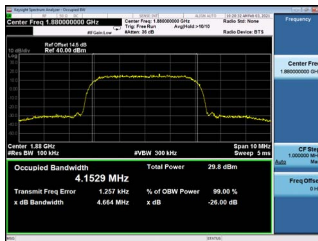
(Plot F2: WCDMA 1900MHz Channel = 9400 Occupied bandwidth)
