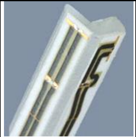
Fig 5.2 Photo of E-field Probe
