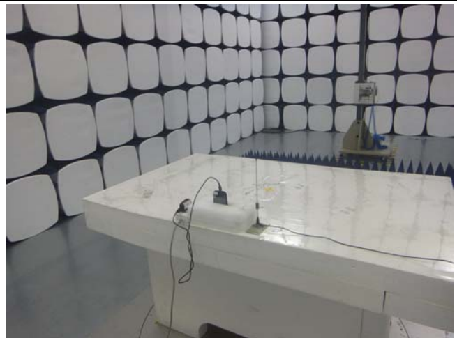
Radiated Spurious Emissions Test Setup Above 1GHz
