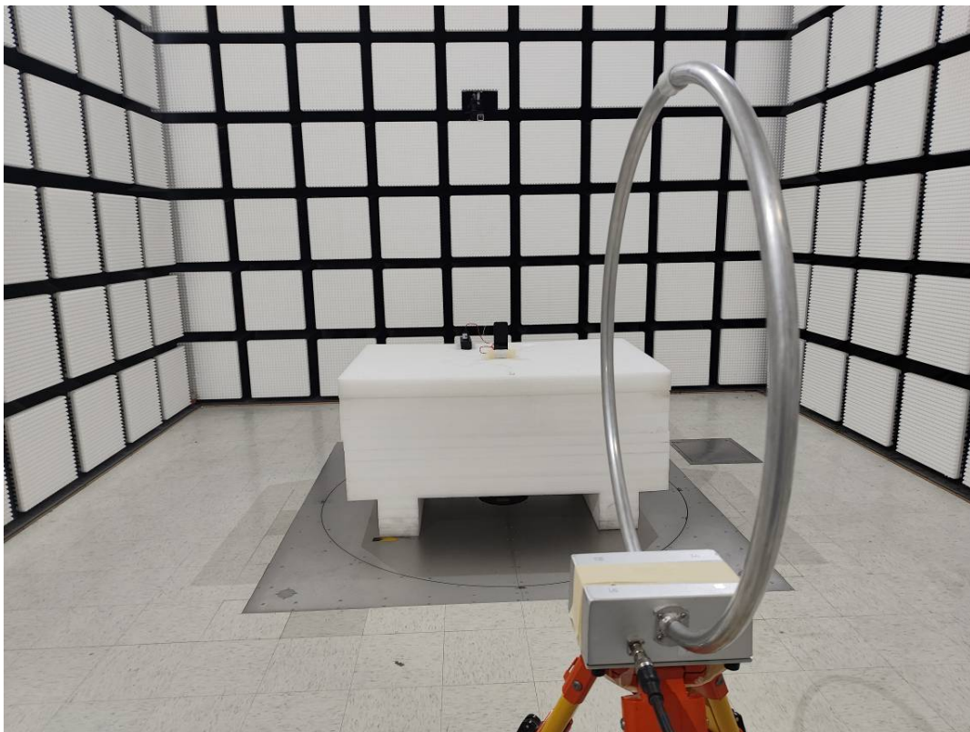
Radiated Emission Below 30MHz View Perpendicular
