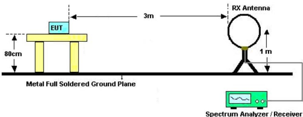
For radiated emission from 30MHz to1GHz
