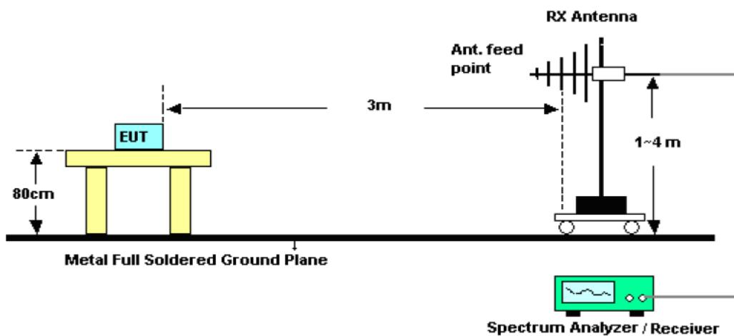
For radiated emission from above1GHz
