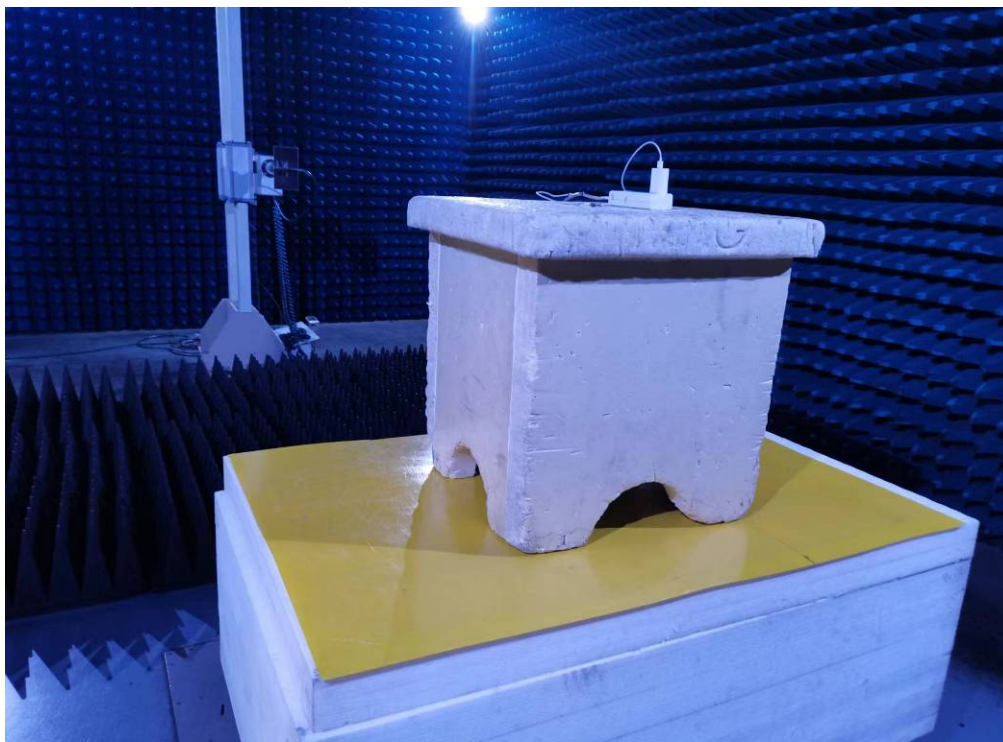
Photo of Radiated Emission Measurement (Above 1G)
