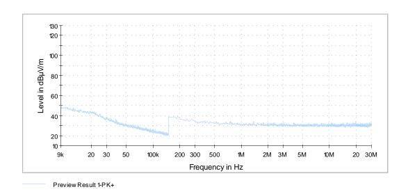
No emissions above the noise floor of the measurement system (max. 49 dB $\mu$ V/m in the frequency range 9 kHz to 490 kHz, max. 34 dB $\mu$ V/m in the frequency range 490 kHz to 1.705 MHz and max. 32 dB $\mu$ V/m in the frequency range 1.705 MHz to 30 MHz (all levels measured with peak detector)) found during the preliminary measurement. So no final measurements on the outdoor test site were carried out.
