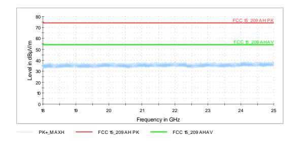
No emissions above the noise floor of the measurement system (max. 38 dB $\mu$ V/m (measured with peak detector)) found during the preliminary measurement. So no final measurements were carried out in this frequency range.
