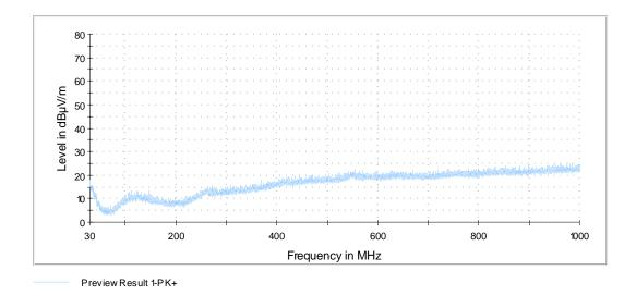
No emissions above the noise floor of the measurement system (max.  $24 \text{ dB}\mu\text{V/m}$  (measured with peak detector)) found during the preliminary measurement. So no final measurements on the open area test site were carried out.
