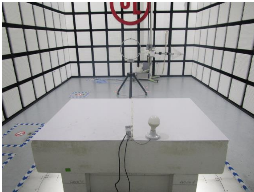
RADIATED RF MEASUREMENT SETUP (Below 30MHz)
