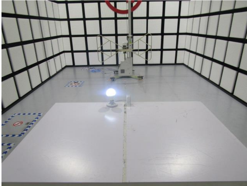
RADIATED RF MEASUREMENT SETUP (30MHz ~ 1 GHz)
