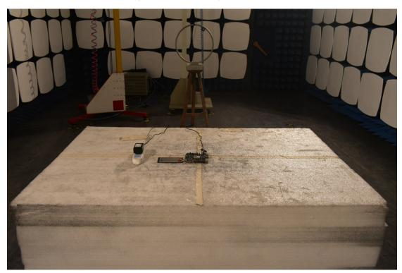
3. Radiated emission (9KHz-30MHz)
