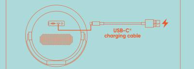
Plug the included USB-C® end of the USB cable into the charging port, and connect the other end of the cable to a power adapter (sold separately). Allow approximately four hours to fully charge the battery.
