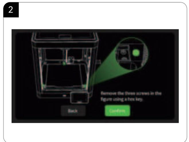
2. Follow the on-screen prompt to remove the three fixed screws of the build platform.
