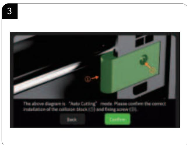
3. Ensure the collision block is correctly installed and click "Confirm."
