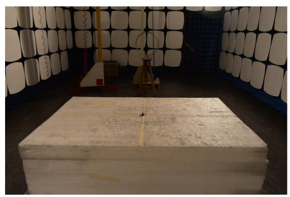
3. Radiated emission (9KHz-30MHz)
