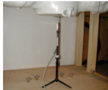
Figure 12.1 Dipole Validation Test Setup
