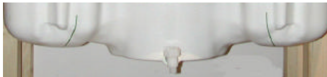
Figure 7.2 SAM Twin Phantom shell
