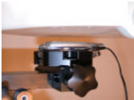
Figure 14.9 Body SAR Test Setup -- w/o Holster --
