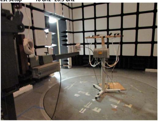
Radiated Test Setup 26.5 GHz - 40 GHz
