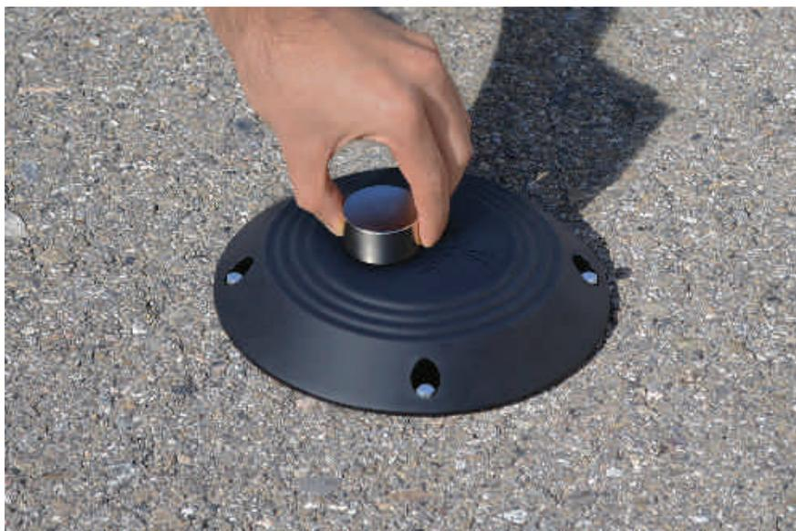
*Figure : Using the magnet to reset the node*
