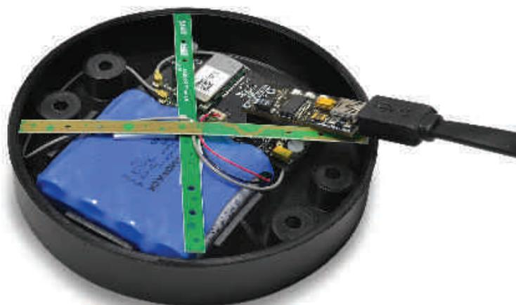
Figure : Plug & Sense! Smart Parking with the USB Programmer tool connected
