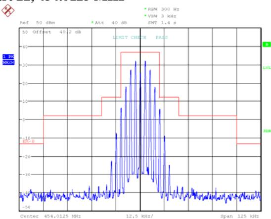
**FCC §2.1051 & §22.861 & §74.462 & § 80.211 & §90.210 - SPURIOUS EMISSIONS AT ANTENNA TERMINALS****Applicable Standard**
