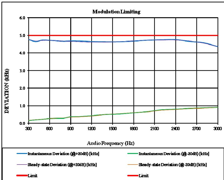
**Audio Frequency Low Pass Filter Response – High Power****12.5kHz:**
