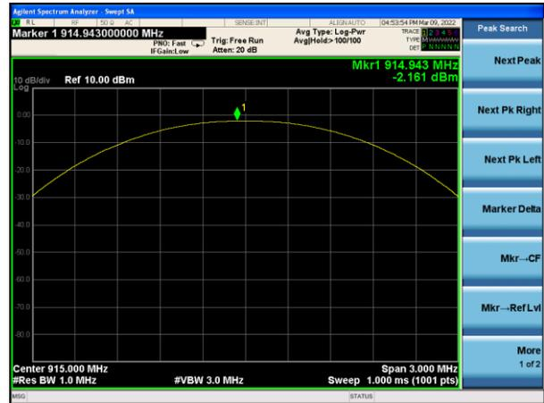
Power spectral density plot on channel 24
