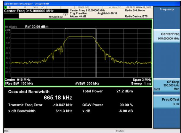
6dB Bandwidth plot on channel 24
