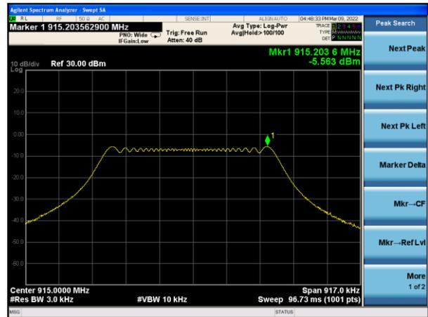
Power spectral density plot on channel 24
