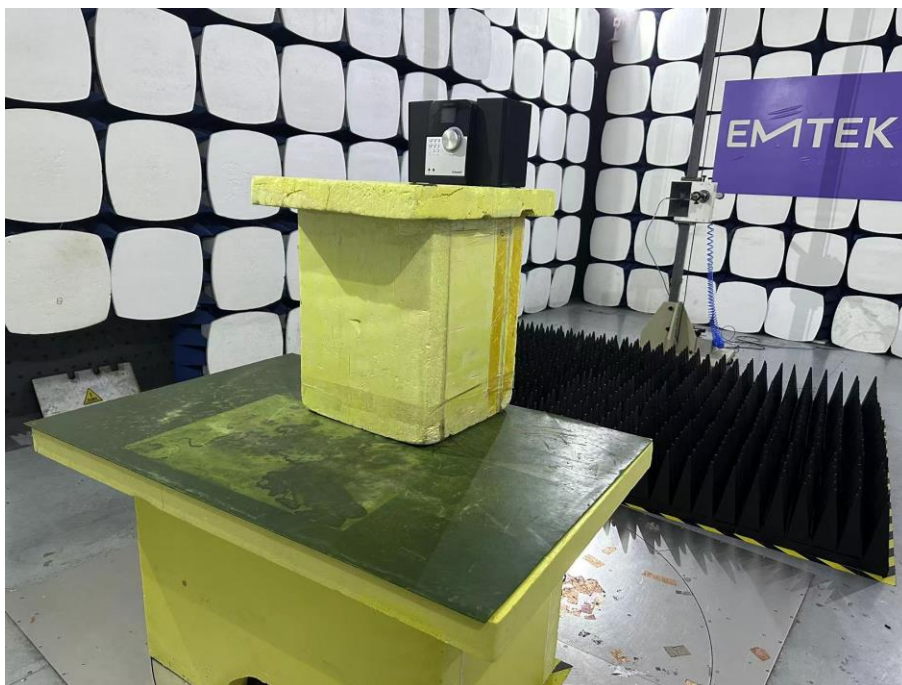
Spurious Emission Test Setup (Above 1GHz)
