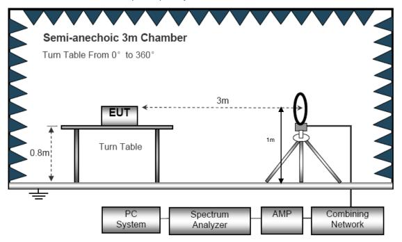
(B) Radiated Emission Test-Up Frequency 30MHz~1GHz
