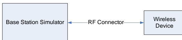
Figure 9-1 Power Measurement Setup
