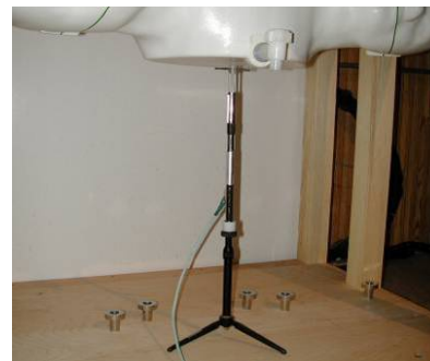
Figure 10-2 System Verification Setup Photo
