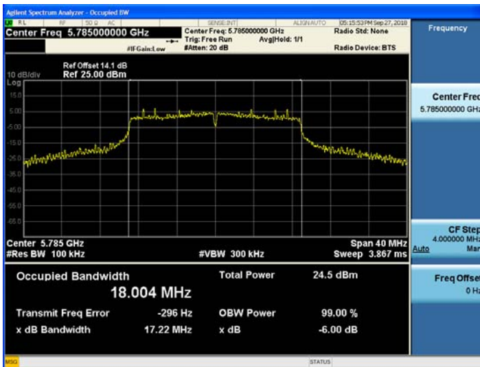
802.11ac_VHT20 UNII 3 BAND 6dB Bandwidth(CH.157)
