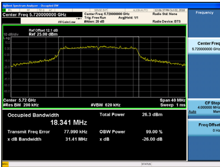
802.11n_HT20 UNII 2C BAND 26dB Bandwidth(CH 144)
