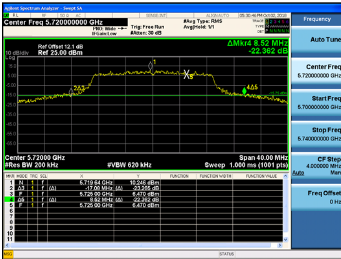
802.11ac_VHT20 CH.144 Bandwidth
