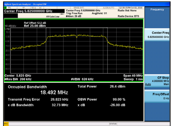
802.11ac_VHT20 UNII 3 BAND 26dB Bandwidth(CH 165)
