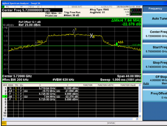
802.11ac_VHT20 CH.144 Bandwidth
