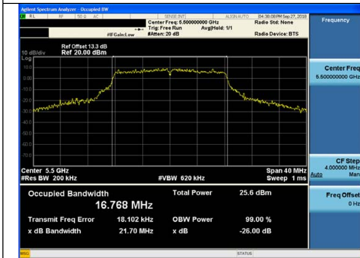
802.11a UNII 2C BAND 26dB Bandwidth (CH 100)
