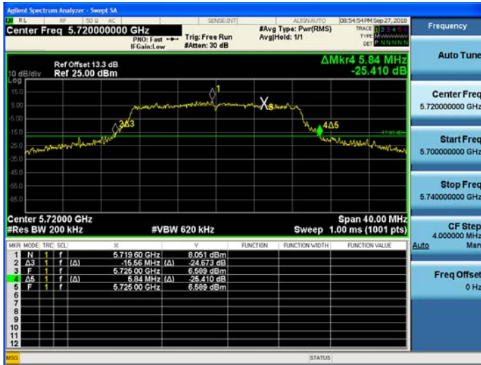
802.11ac_VHT20 CH.144 Bandwidth
