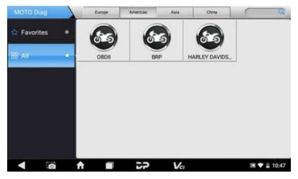
The following takes OBD II as an example to introduce how to start the diagnosis. Click the OBD-II Engine icon under the menu
